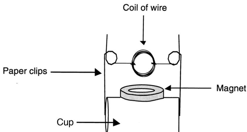
7. Clip one alligator clip to each of the paper clips and hook the other end to the battery.
