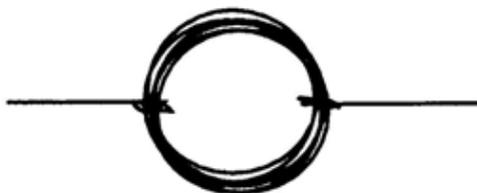
**\*\*NOTE:** The loop must be even and the end wires as straight as possible so that the coil will spin evenly. If the wires are unbalanced, the coil will be weighted down on one side.
