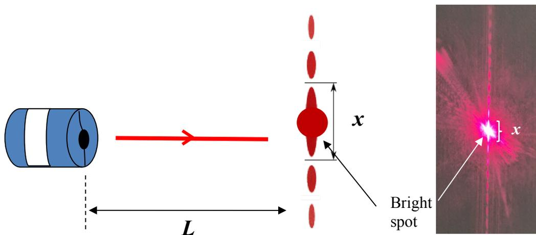
4. Measure (in cm) the width of the central bright spot. That is, measure the distance between the **centers of the dark bands** on either side of the central bright spot.
