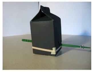
2. Orient the milk carton near the edge of the table such that it is pointed in a direction with at least 3 meters of open floor space. Use a piece of masking tape to mark off the point of the floor in line with edge of the table from which the projectile will be launched. Lay down the meter stick or tape measure on the line along which the chopstick will be launched. If you're using a meter stick, mark off three 100-cm increments with masking tape to save yourself time later.
