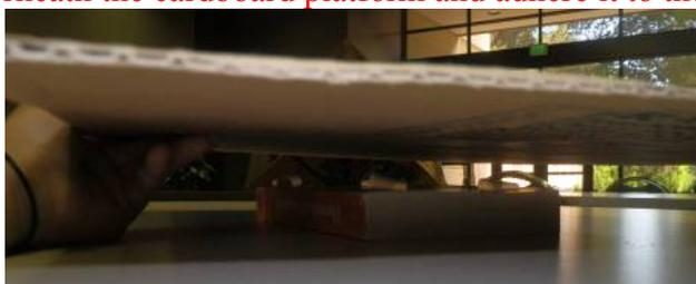
Center a sheet of paper on the upper side of the cardboard platform, so that it completely covers the unseen object underneath, and tape this sheet down to the cardboard.
